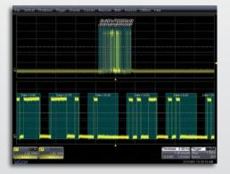
The serial data trigger will quickly isolate events on a bus eliminating the need to set manual triggers and hoping to catch the right information. Trigger conditions can be entered in binary or hexadecimal formats and conditional trigger capabilities even allow triggering on a range of different events.
