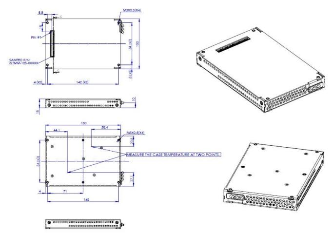
To the EDFA box a Heat-sink will be connected. Thermal paste will be added between amplifier and Heatsink to assure good thermal connectivity.
