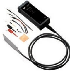
The ZS Series probes provide high impedance and an extensive set of probe tips and ground accessories to handle a wide range of probing scenarios. The high 1 M $\Omega$  input resistance and low input capacitance mean this probe is ideal for all frequencies. The ZS Series probes provide full system bandwidth for all Teledyne LeCroy oscilloscopes having bandwidths of 4 GHz and lower.
