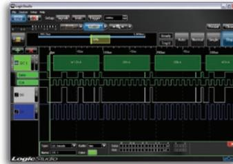
View decoded protocol information for I<sup>2</sup>C, SPI and UART busses plus trigger on data being transmitted on the serial busses.
