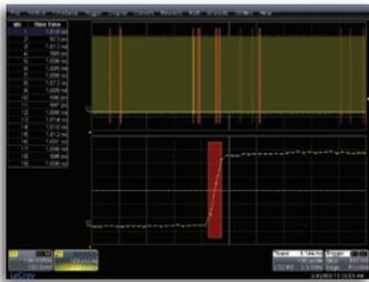
Use WaveScan to search for and identify anomalies on analog or digital signals.
