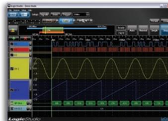
Turn any PC into an MSO by connecting LogicStudio to any of ten popular oscilloscopes from Teledyne LeCroy, Tektronix and Agilent.
