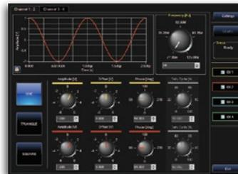
Quickly generate basic functions like sine, square and triangle waves with a dedicated user interface.
