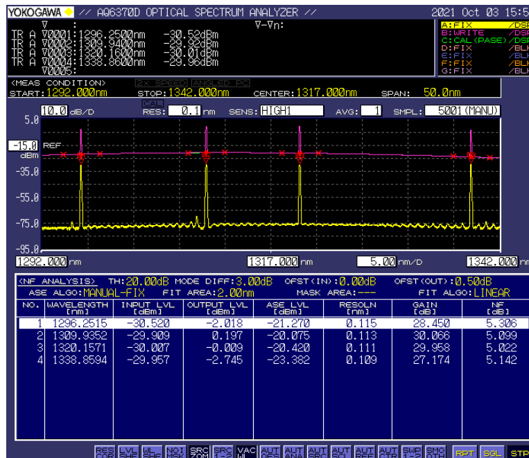
Optical gain and NF for 4 wavelengths input
