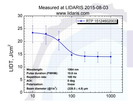
Typical laser damage curve of AR-coated RTP substrates:
