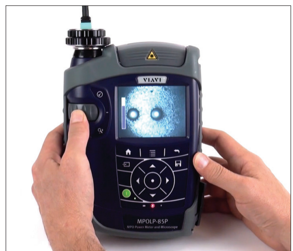
MPO connector inspection with the integrated PCM
