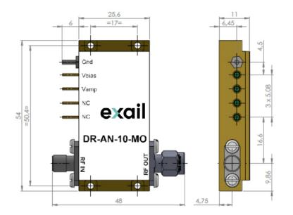
The heat-sinking of the module is necessary. It's user responsability to use an adequate heat-sink. Refer to page 5 for Exail recommended heat-sink.
