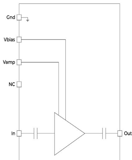
**Mechanical Diagram and Pinout**
