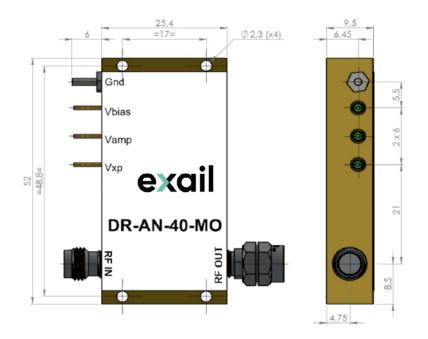
The heat-sinking of the module is necessary. It's user responsability to use an adequate heat-sink. Refer to page 5 for Exail recommended heat-sink.
