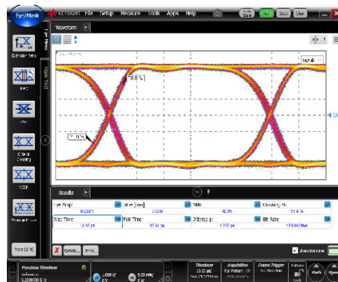
Output response Eye amplitude = 6 V_{\text{pp}}
