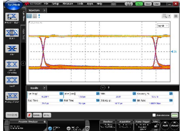
Data Rate = 1 Gb/s, V_{in} = 220\text{ mV}_{pp}
