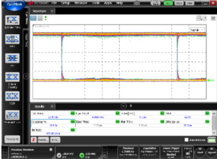
Eye Diagrams - 10 Gb/s - 1310 nm
