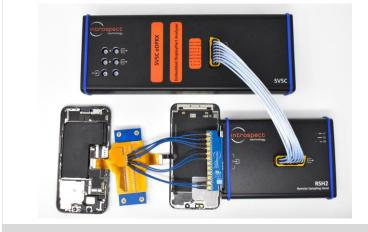
The RSH2 and SV5C-eDP Analyzer setup to probe an Embedded DisplayPort design
